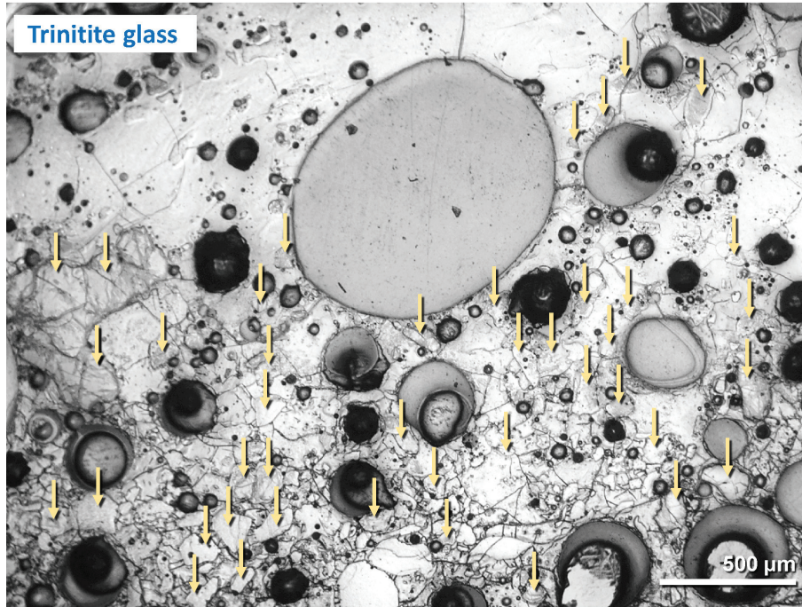
Figure S3: Shock-fractured quartz grains in Trinity meltglass. Epi-photomicrograph of a thin-sectioned slide. We analyzed 42 grains (arrows) with shock fractures from ejected meltglass at a concentration of ~700 quartz grains per cm 2 .
