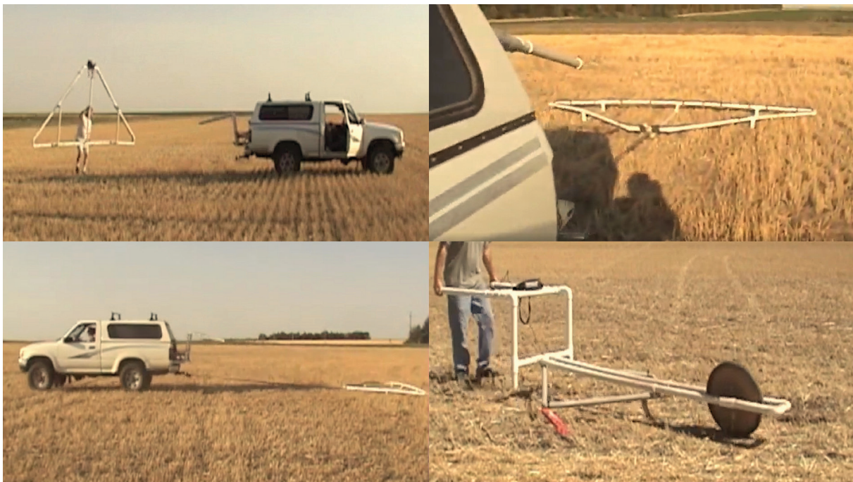
Figure 4: Magnetometer survey conducted in a gridded search pattern with a raster scan and a 30 cm overlap of a survey area. Note the complete absence of impact surface features.
