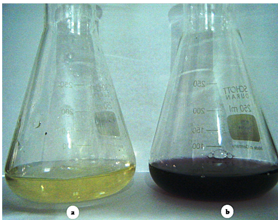
Fig. 1. Reaction of aqueous A. indica leaves extract with 1 mM \text{HAuCl}_4 solution. (a) Leaves extract alone; (b) pinkish violet colour formation after the addition of 1 mM \text{HAuCl}_4 solution at 30 min of incubation.
