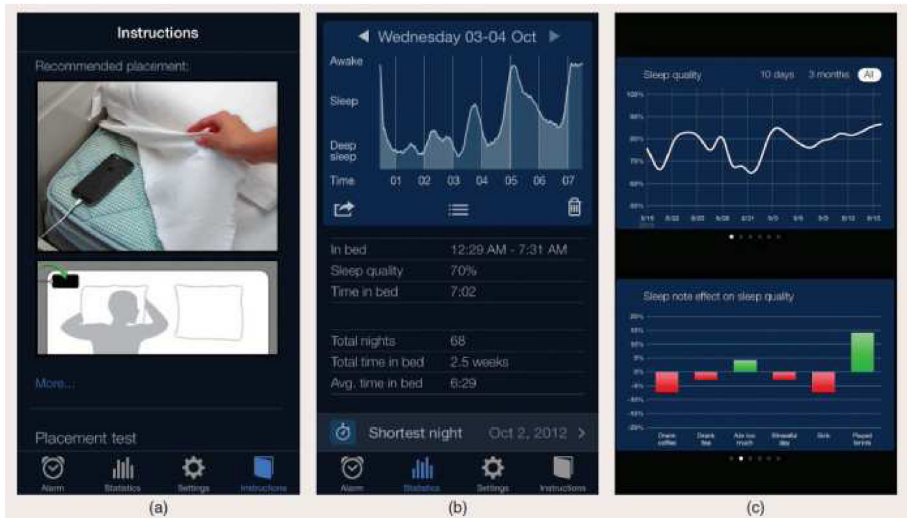
Figure 3. Smartphone applications to track sleep without external sensors. Smartphone applications use movement patterns in order to detect sleep, sleep disorders, and sometimes even sleep apnea 21 . Here, we present the screenshots of a simple app which tracks sleep depth and, based on this, derives sleep duration and a kind of sleep quality. Frame (a) shows how the smartphone should be used (placed underneath the blanket). Frame (b) shows the report of a single night with a trace reflecting activity and estimating sleep depth. Frame (c) shows the sequence of several nights summarized and with that a tracking of sleep quality over one week or a longer time period. Unfortunately, most sleep apps similar to this one have not been checked against a sleep recording or validated clinically and scientifically. They remain to be gimmicks for lifestyle use.
