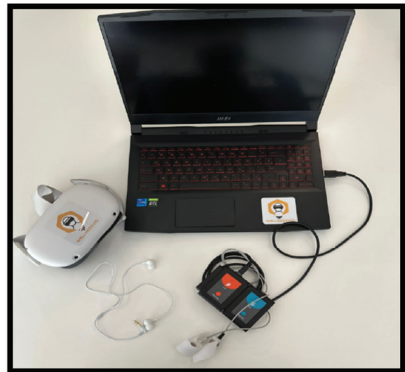
Figure 2: Oculus Quest 2 VR headset and GSR connected to the laptop. Abbreviations: GSR, galvanic skin response; VR, virtual reality.
