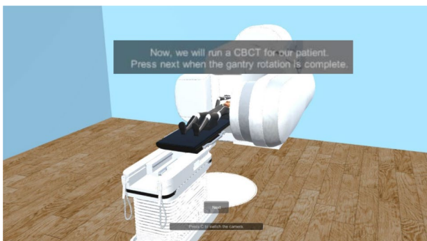
Fig. 14 Treatment Delivery Simulation Scene - CBCT - The patient undergoes a CBCT on the first treatment, and once a week to validate the positioning of his tumor in the center of our Radiotherapy plan. Here, you may see the extended kV source (above the patient) and detector (under the table), taking images between 0° and 180° for CT reconstruction
