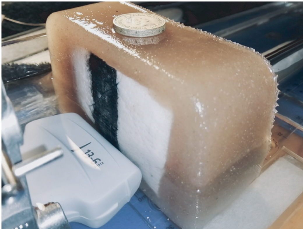
Figure 5 Experimental setup of the probe sonicating tattooed pork embedded in a tissue-mimicking phantom. According to practice [35], a St Helena £1 coin, with a diameter of 23.44 mm and thickness of 2.80 mm, has been added for scale and for three-dimensional perspective. The dimensions of the phantom were 112×79×40 mm 3 .
