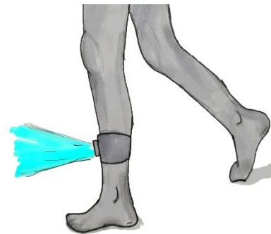
Figure 1: Sketch of the motion sensitive lighting wearable illuminating as the wearer stops moving
