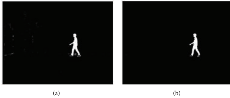
FIGURE 6: Resultant foreground image. (a) Foreground with random noise (b) Postprocessed foreground image.
