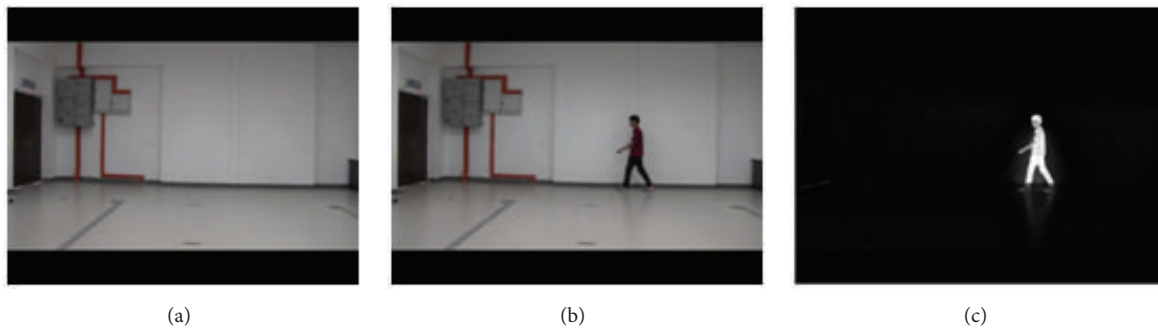
FIGURE 3: Process of object extraction. (a) Empty background frame. (b) New frame with walking subject. (c) Difference image.
