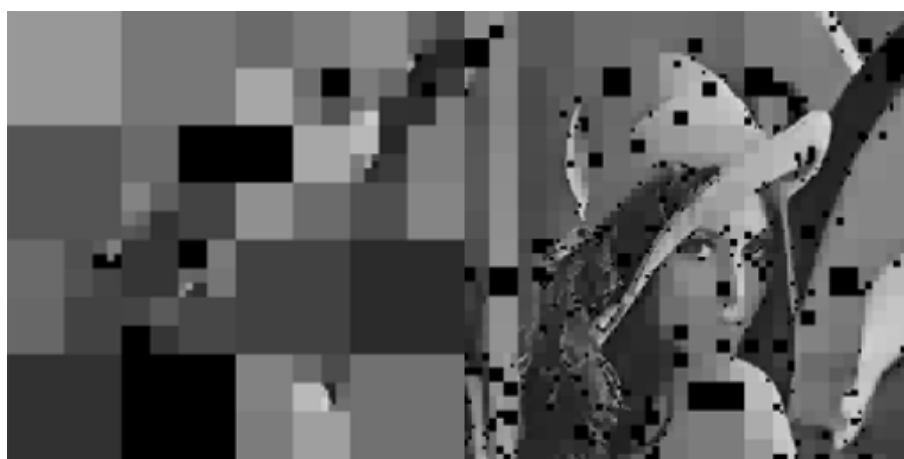
Figure 22. Initial Transmitted Image Frame ( t = 0 s—left side)—Converged Transmitted Image Frame ( t = 225 s—right side) under 10% Network Congestion.
