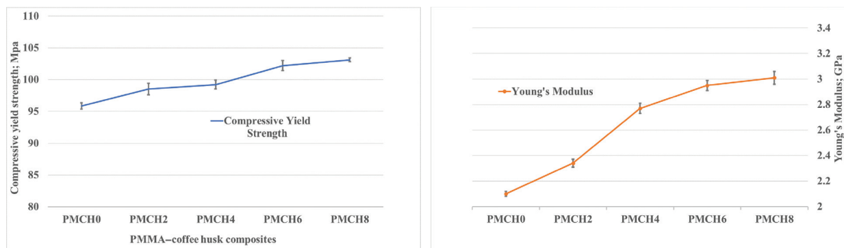
Figure 4: Compressive yield strength and Young's modulus of PMMA-CH composites. Abbreviation: PMMA-CH, polymethyl methacrylate-coffee husk.
