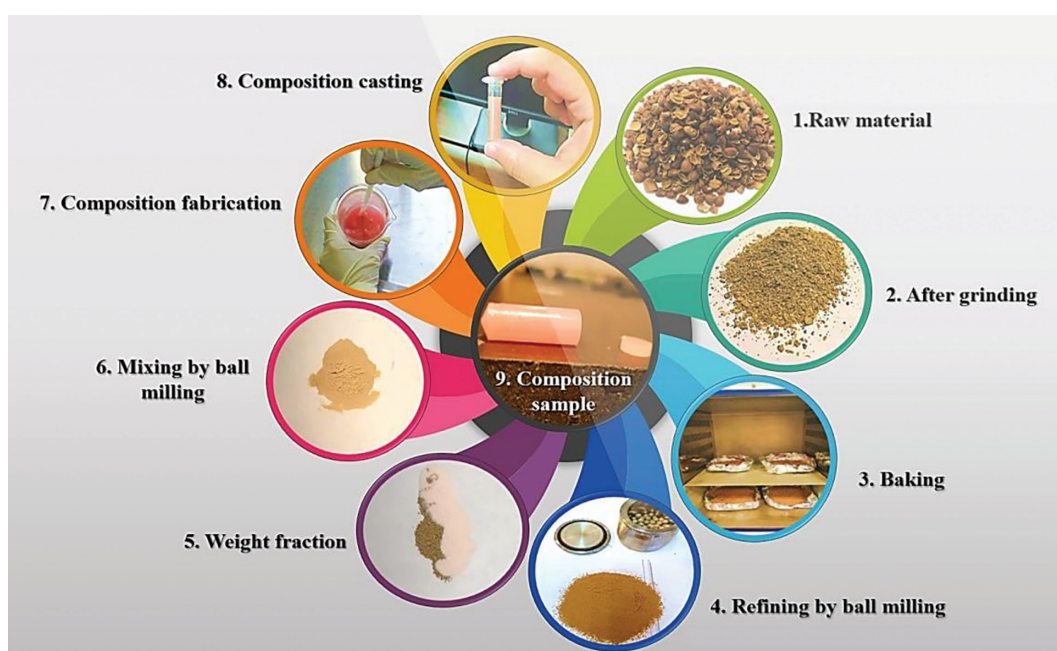
Figure 1: Flowchart of polymethyl methacrylate-coffee husk composite sample preparation.
