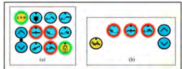
Figure 18. (a) Attendant and (b) nurse control panels have three buttons (BACKREST, LIFT and THIGH buttons) in common (circled in red). Nontrivial buttons (CPR and LOCK buttons) are located on the attendant control panel (circled in green).
