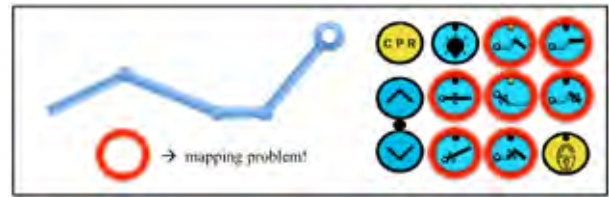
Figure 7. User's workload is increased due to bad mapping of images on attendant control panel (buttons circled in red) located on one of the sides of the bed (simulation snapshot).
