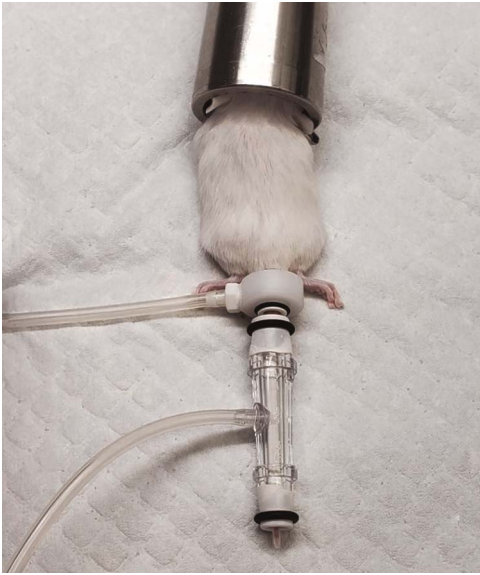
Figure 8: Indirect blood pressure measurement. Blood pressure can be monitored indirectly with equipment, such as with the Kent Scientific CODA Monitor System, which uses a tail-cuff to monitor the indirect blood pressure.
