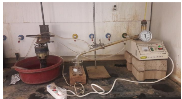
Plate (31): Semi-batch reactor pieces of equipment
