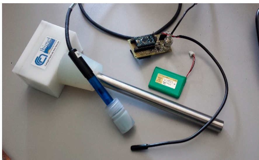
Figure 3. WineDuino node with sensor and dipstick.
